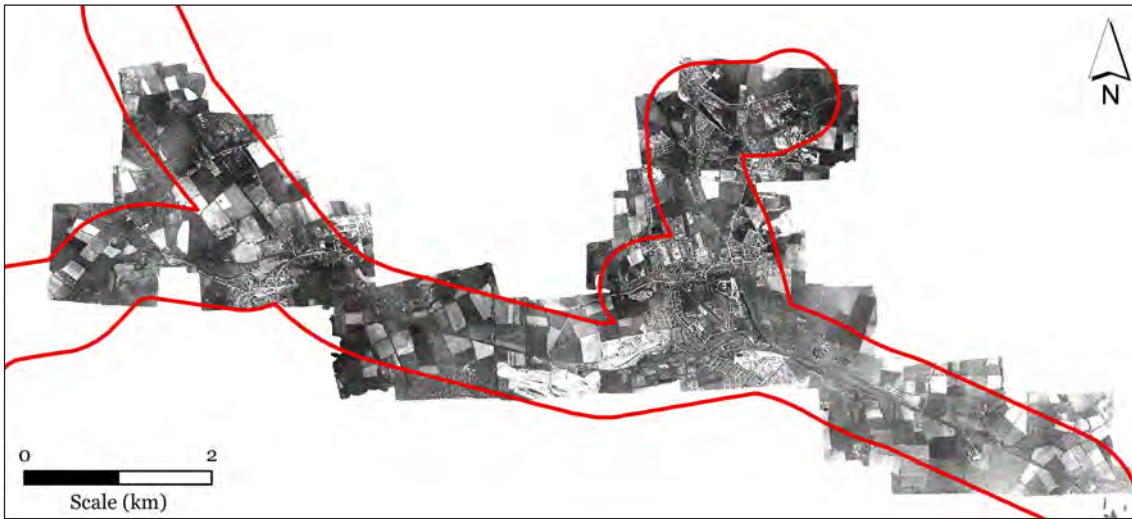
Fig 83: A large portion of the western half of the railway was mapped from one single sortie of RAF photography, mosaicked and georeferenced using Structure from Motion. SfM RAF/58/B/37 V 5029-5379 17-MAY-1948 Historic England Archive (RAF Photography).
