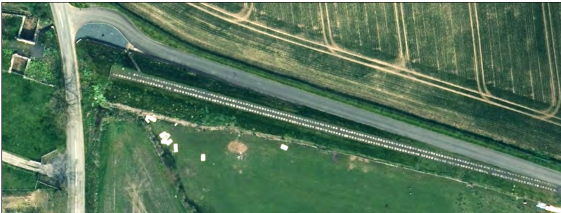
Fig 81: Where the S&DR spanned Brusselton Lane is the only place in the project where the original stone sleepers were visible on aerial photographs. They were exposed recently by a local volunteer group and are not visible on historic aerial photography. Detail of NZ2125 06-MAY-2016 © Bluesky International/Getmapping PLC.
